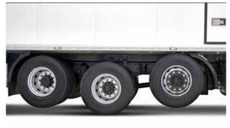
For vehicles with 6x2 and 8x2 axle type, in unloaded conditions, the rear axle is off the ground. This mechanism avoids unnecessary tire wear. When the vehicle is stopped for loading, tires automatically drop down, thanks to the Auto-drop feature.
