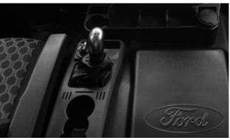
12-speed automated transmission is provided as an option for 420 PS vehicles. The system selects the most appropriate gear for each situation automatically and provides great comfort. Intarder
