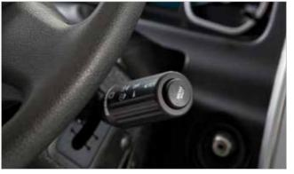
The 600 KW Intarder, which is available as an optional feature on vehicles, meets all expectations under such challenging conditions as going downhill while loaded. Preventing unnecessary use of your service brake, it prolongs service life.
