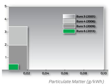
Euro 6 standards allow exhaust emissions at one-fifth of Euro 5 standards. The Euro 6 testing procedure also involves counting exhaust particulates.
