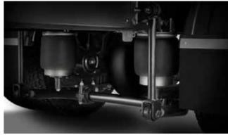
The newly developed rear air suspension is developed for the 4x2 and 6x2 models. In addition to the unique driving comfort, it guarantees much safer transport of fragile loads.
