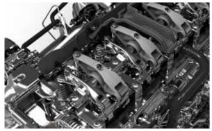
The new integrated engine brake, available as standard equipment, provides additional 340 kW brake power for 420 PS vehicles and 220 kW for 330 PS vehicles. This high brake power can be applied gradually, meeting varying braking needs according to load conditions.
