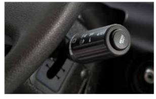
The 600 KW Intarder, which is available as an optional feature on 420 PS vehicles, meets all expectations under such challenging conditions as going downhill while loaded. Preventing unnecessary use of your service brake, it prolongs service life.
