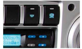
Supporting efficient use of the engine brake and the Intarder, the Smart Brake Management System, which can be activated by using the button on the front panel, makes best use of makes the best use of the auxiliary brakes based on braking requirements and ensures that service brakes are always ready for emergencies.
